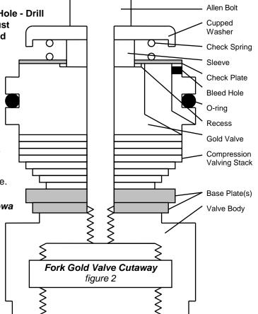
some of the original shims or an additional spacer on the shaft below the base plate. Be sure that the spring cup is straddling the step!!!
